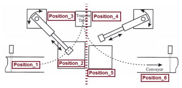
**Figure 3**: Specific positions for each robot arm. During the process, it is assumed that both robots are positioned at Position\_3 and Position\_4 at the start of the process for Robot\_Arm\_1 and Robot\_Arm\_2 respectively.
