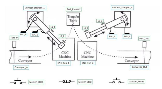
**Figure 2**: Possible system setup with limit switches and pneumatic cylinders attached to stepper motors. Blue square items are outputs, green square items are inputs
